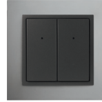
WSB3-40, WSB3-40H Four button controller, built-in temperature sensor and humidity (version H), 2x AIN/DIN, 2x indication LED, comes in LOGUS 90 design.
