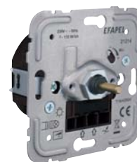
21214 Dimmer/two-way switch for energy saving lamps - 110VA R, L 7 - 110W/VA. Dimming LED.
